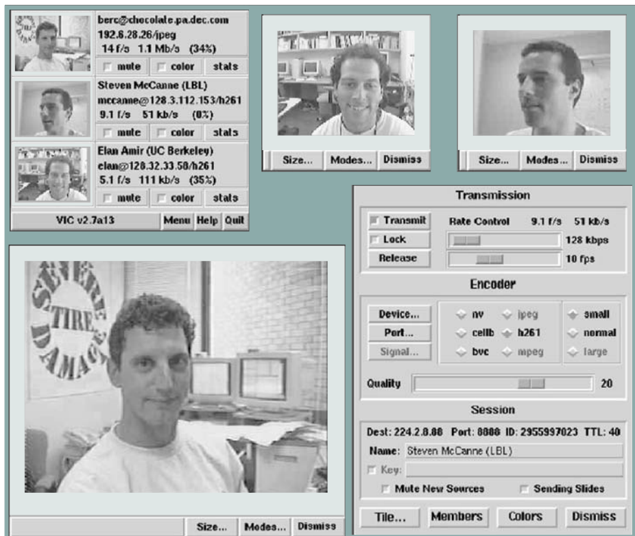
Figure 1.1 The vic video application. This shot is from a 1995 release of the tool.
