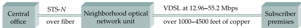
Figure 2.6 VDSL connects the subscriber to the optical network that reaches the neighborhood.
